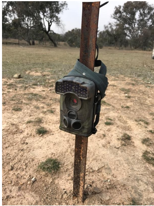
Figure 3.4: A motion sensor/thermal camera (Ltl Acorn brand – Model Ltl-5310A) (Image: Author's own)
